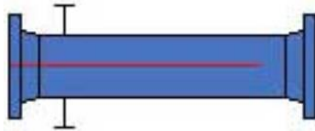
two pass shell with longitudinal baffle
